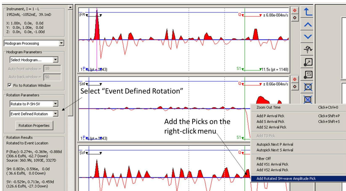
Figure 7-11: The user interface for manual picking P-, SH-, and SV-wave amplitude used in moment tensor inversion.
