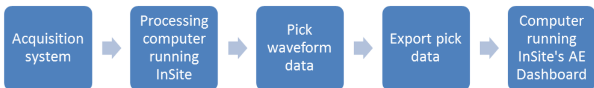
Figure 19-3: Flow chart of acquiring data to displaying data on the dashboard
