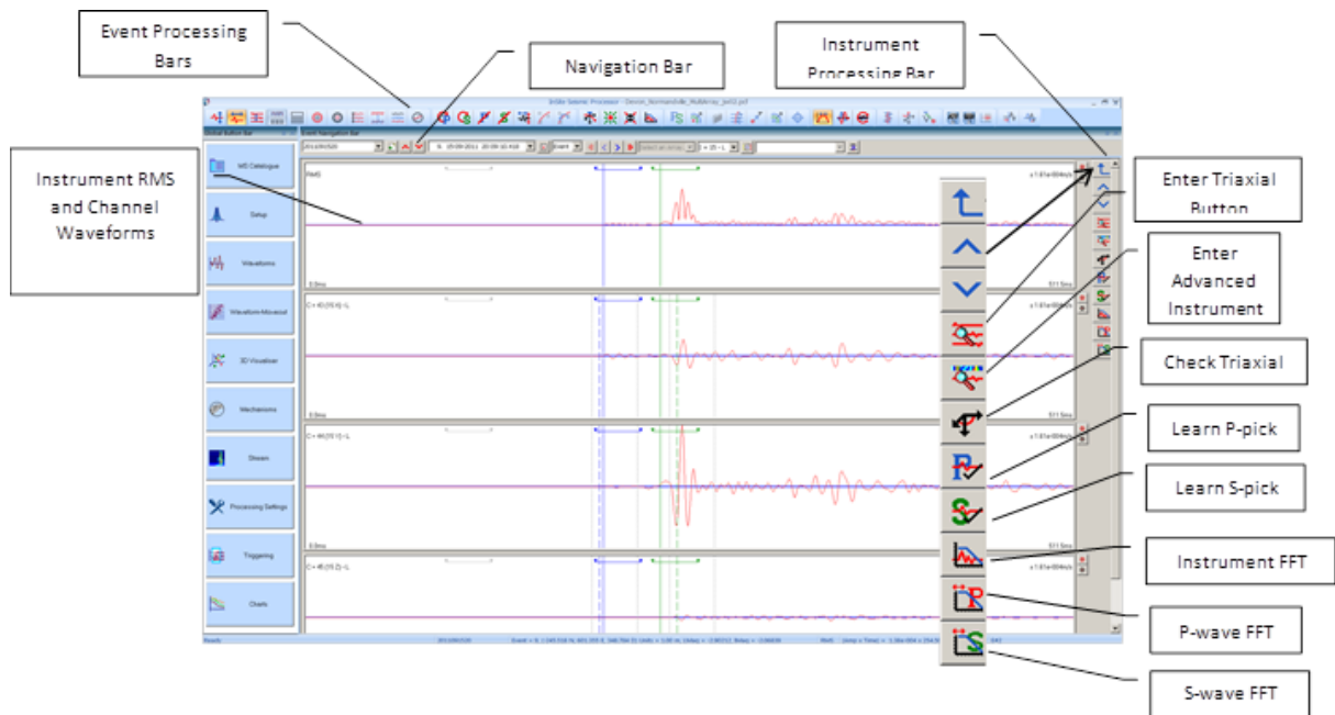
Figure 7-3: The Instrument View in the Waveform Visualiser for a correctly configured triaxial instrument. Clicking on the Enter Triaxial button will open the Advanced Waveform Visualiser. Clicking on the Enter Advanced Instrument button will open the Advanced Instrument Visualiser.
